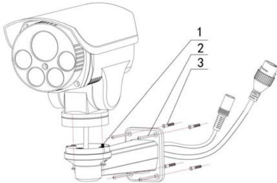
**Bracket Mounting** - The first thing to fasten the bracket supplied separately to the camera body with the two screws provided (1). The cables pass through the bracket and protruding rear.
